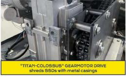
The Kobra DIGITAL-PRO is eqipped with the "Titan-Colossus" gearmotor drive specially designed heavy duty cutting knives with unmatched power to shred large quantities of: SSDs (also with metal casings), smartphones, SIM cards, USB drives, flash memory, IC chips, Credit Cards with chips, PC Boards, CD/DVD/BD.
